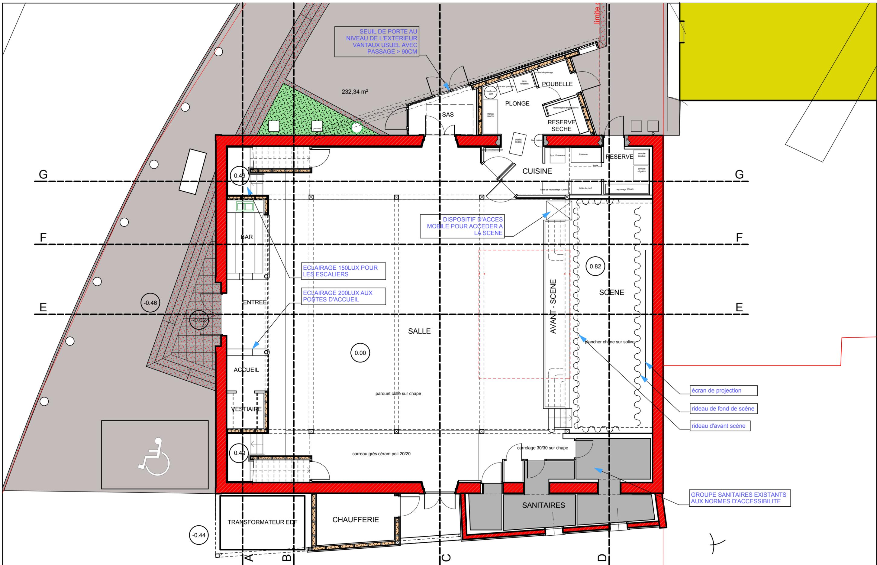
SEUIL DE PORTE AU NIVEAU DE L'EXTERIEUR VANTAUX USUEL AVEC PASSAGE > 90CM
